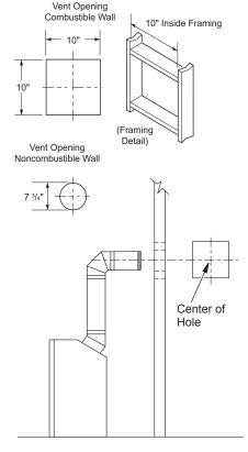
Figure 9 - Vent Opening Requirements
